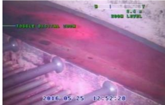
Fig. 5. Figure on the left is the dye penetrant application unit with a dye and flush lance attached to a remote camera. Figure on the right is the top of the steam tube bundle with dye penetrant on the surface before flushing.
