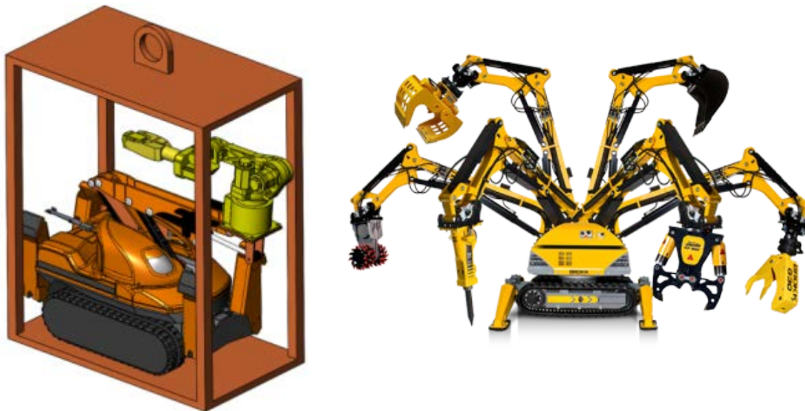
Fig. 10. Figure on the left shows a model of the BROKK 100 with the KUKA arm attached to the robot on the lifting mechanism that will lower and raise the unit out of the cell. Figure on the right shows a typical BROKK 100 with some of the other attachments that are readily available for the BROKK if needed.
