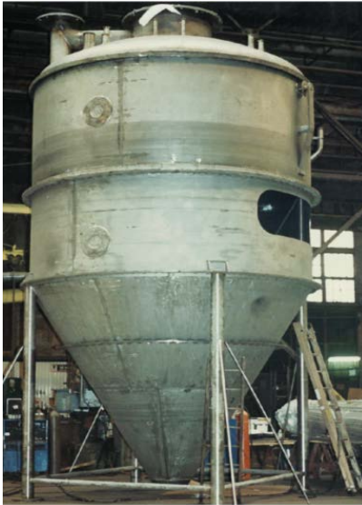
Fig. 3. Construction of 25H Evaporator Vessel
